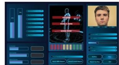
All settings can be done remotely using this software. Real time WTMD's can be screened. Recordings can be made on a hard disk. Usage with an optional kiosk is possible. Face image photos can be taken and saved with date and time information.
