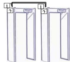
Do not forget to turn OFF the switch on the main board of the slave WTMD. See Section 6.13
