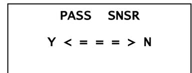
The pass sensor in s3/s6 is underneath the Control Unit and it is a one way counter. Using **UP&DOWN** buttons select (with the **SEL** button) **"Y"** to activate the Pass Sensor, select **"N"** to deactivate it.
